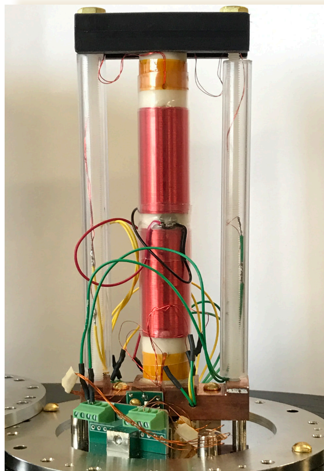
Fig. 1: The Hartshorn coil for measuring magnetic susceptibility, mounted on the temperature-controlled baseplate of the TeachSpin CMP dewar (shown with inner and outer vacuum cans removed, and with the dewar inverted).
